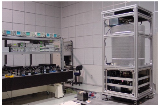
Figure 2. The cesium atomic fountain primary frequency standard (NICT-CsF1).
