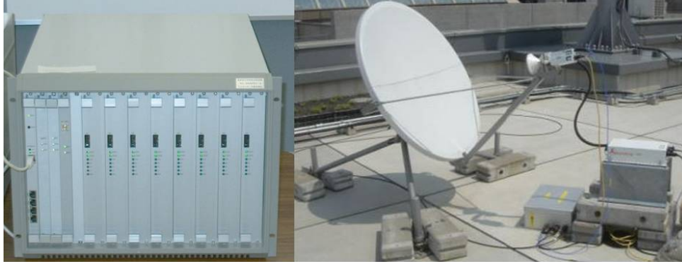
Figure 5. TWSTFT: NICT multi-channel modem and portable station.
