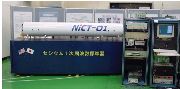
Figure 1. Optically pumped cesium primary frequency standard (NICT-O1).
